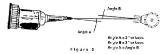
The important thing is that the two center lines are parallel, and that the angle of them to the driveshaft isn't too large, 3 degress max according to the photo above.
