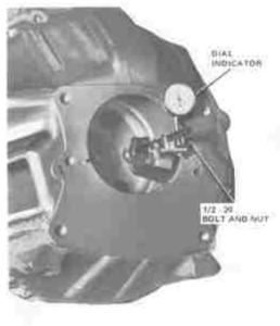
transmission to the bellhousing and the fit of the pilot bushing to the transmission input shaft.
