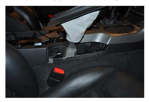
Remove the two 7mm screws that were exposed when the E-Brake boot was moved out of the way (shown below).
