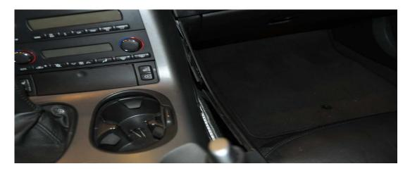
Lift the back of the center console off of the studs in the rear and slide it back towards the rear of the car. It may take some maneuvering to get it around the E-Brake boot.
