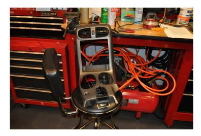
This is what you're left with in the car. If you want to remove the radio and the A/C head unit just remove the six 7mm bolts and pull them out. You'll have several wiring harnesses in the back to disconnect as you go but there is plenty of slack in all of them. I didn't get pictures of this step but it's pretty intuitive.
