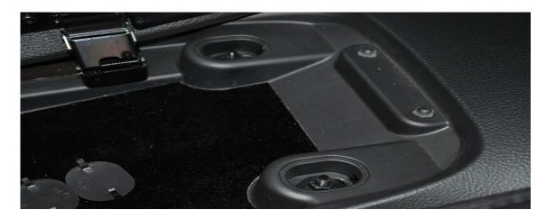
Using a wrapped flat blade screwdriver pry up on the oval shaped plastic trim piece at the front of the center console as shown. Note: If you have the F55 suspension option you'll have a wiring harness to disconnect underneath the oval piece.
