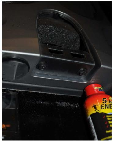
Pull up on the passenger side of the E-Brake boot. There are three clips that hold the boot down that you'll have to pop loose. Do so carefully and pull the E-Brake boot up as shown.
