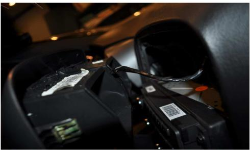
Once you've disconnected the connectors at the back of the bezel rotate it so the top of it goes toward the passenger seat and disconnect the remaining two wiring harnesses toward the back of the piece. The Active Handling/Traction Control connector is pretty much self explanatory. There is a plastic piece on the side of it that you gently pry up that will allow you to disconnect it.
