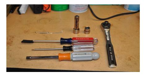
Flat blade screwdriver with some electrical tape wrapped around the blade (to protect the plastic pieces).
