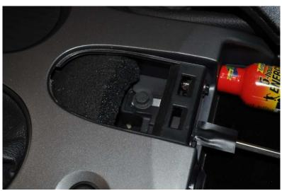
Remove the 10mm bolt that is underneath the oval shaped trim piece.
