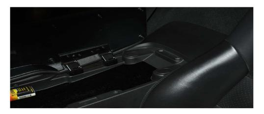
Remove the two 10mm nuts that were under the caps at the rear of the center console.
