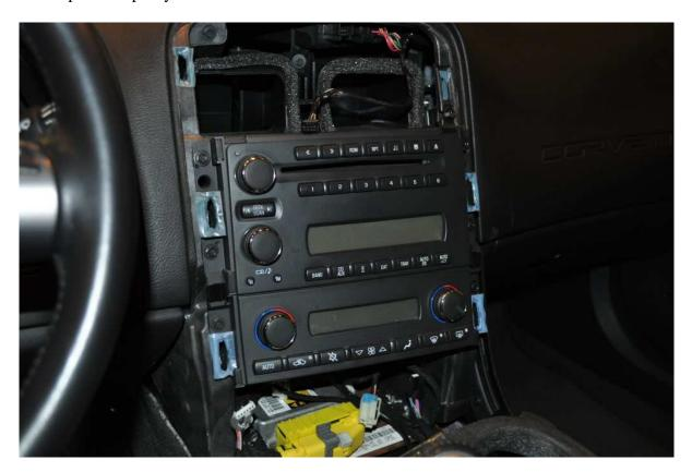
Reverse the steps above to get everything back together. Don't forget to reconnect the hazard switch at the top of the bezel... that one's easy to forget.
