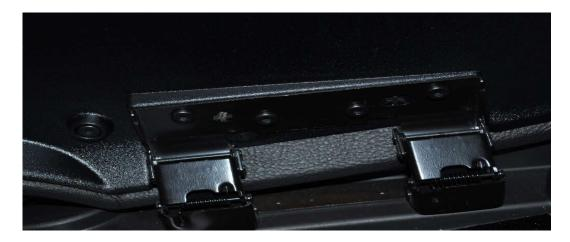
Using either your fingernails or a wrapped flat blade screwdriver remove the plastic caps at the rear of the center console.
