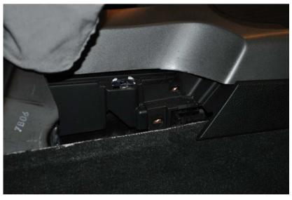
Carefully loosen the plastic trim piece that follows the radio bezel on the passenger side of the car. You don't need to take it all the way off, just loosen it as shown.
